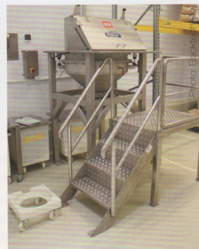
Left photo: Two tanks provide for the sufficient oil quantity that is transported via a pump to the dough preparation unit and the kneader. Right photo: The small-quantity ingredients as well as flour and sugar must be sieved prior to processing to exclude pollution.
