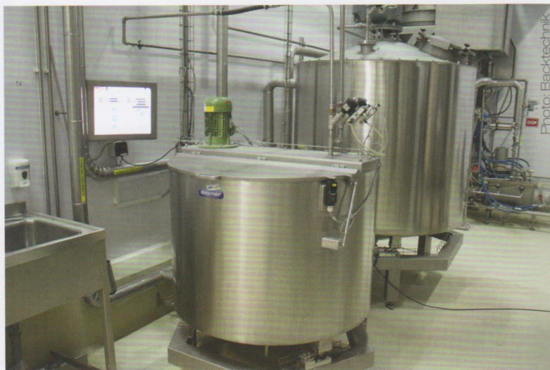
Left photo: The 30-ton sugar silo and the three 50-ton flour silos are located outside the bakery. The flour for the production is delivered by a mill that belongs to the group. Right photo: At first, the yeast is dissolved and after that, it is pumped to the storage tank next to it.
