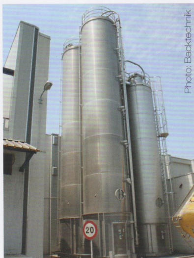
Left photo: The 30-ton sugar silo and the three 50-ton flour silos are located outside the bakery. The flour for the production is delivered by a mill that belongs to the group. Right photo: At first, the yeast is dissolved and after that, it is pumped to the storage tank next to it.
