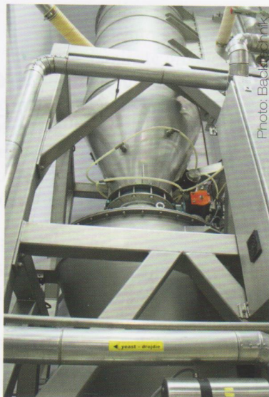
Left photo: While the flour is continuously filled to be mixed in the lower scale, the next batch can be weighed in the upper scale. Right photo: Daxner International has also delivered the plant system for weighing the product above the Turkington kneader.
