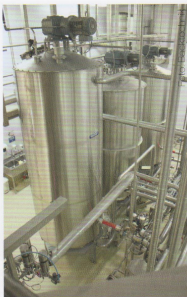
Left photo: The starter dough gets the time to develop in two maturity containers. The big cooled storage tank is on the left. Middle photo: Before the starter dough flows into the storage tank, it is cooled down to 5°C in a plate heat exchanger. Right photo: An extensive cooling system ensures that the individual ingredients are at the desired temperatures.
