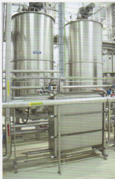
Left photo: The starter dough gets the time to develop in two maturity containers. The big cooled storage tank is on the left. Middle photo: Before the starter dough flows into the storage tank, it is cooled down to 5°C in a plate heat exchanger. Right photo: An extensive cooling system ensures that the individual ingredients are at the desired temperatures.
