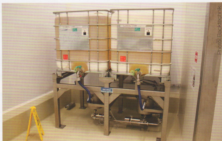
Left photo: Two tanks provide for the sufficient oil quantity that is transported via a pump to the dough preparation unit and the kneader. Right photo: The small-quantity ingredients as well as flour and sugar must be sieved prior to processing to exclude pollution.
