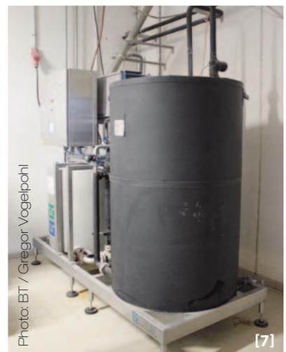
[5] Liquid yeast (right) and the finished creamy mass made from bread residue and water are stored in the two tanks. [6] Dough residue from production is first mixed with water and then added to the pre-dough mixer. [7] The brine has a temperature of approximately -7 °C so that no flaked ice is required for most doughs.
