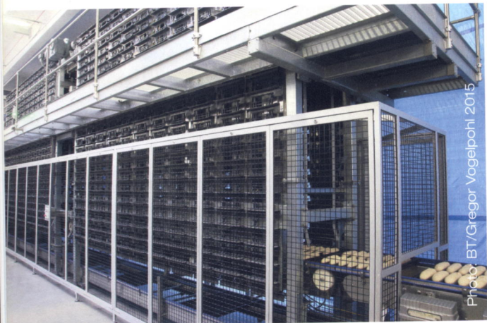
To cool down the pastry to the desired temperature, a capacity of 308 baking plates is planned in the MVS cooling tower.
