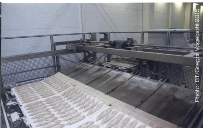
The loader with open conveyor belt will be driven by chains and chain wheels. It takes the products from the peel boards and then, it puts them into the stone tunnel oven.
