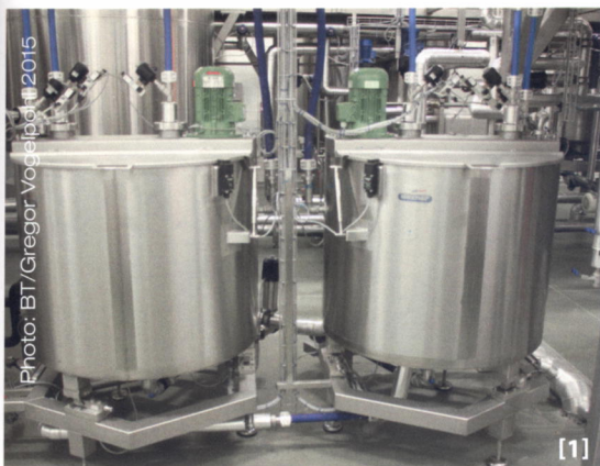
[1] Yeast is solved, cooled and exactly dosed into the dough mixing unit for the wheat starter dough. [2] The components of the wheat starter dough are continuously added into the dough preparation unit and conveyed to the mixing screw via the connections. Then, the mixing screw generates a homogeneous mass. [3] The seeds and the grains are compiled for the yeast-free sponge and added into the tank via the two sack emptying machines.
