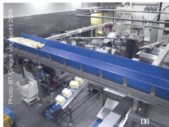
[1] Yeast is solved, cooled and exactly dosed into the dough mixing unit for the wheat starter dough. [2] The components of the wheat starter dough are continuously added into the dough preparation unit and conveyed to the mixing screw via the connections. Then, the mixing screw generates a homogeneous mass. [3] The seeds and the grains are compiled for the yeast-free sponge and added into the tank via the two sack emptying machines.
