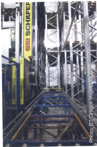
The new fully automatic storage has a capacity of 20,000 pallets and is well protected from fire due to its reduced constituent part of oxygen.
