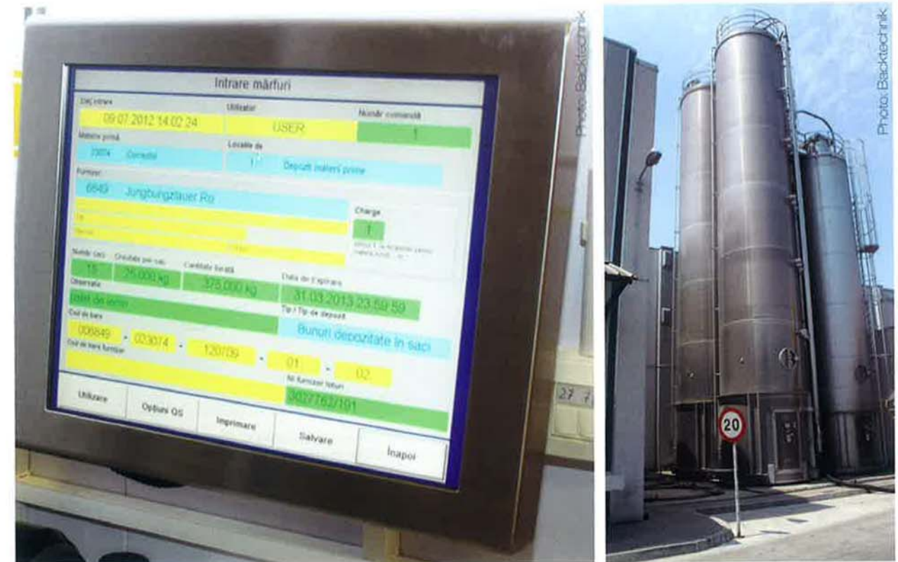
Left photo: One employee enters all raw materials into the warehouse management system of the raw materials warehouse and allocates bar codes that are scanned when the ingredient is transferred to the production process. Right photo: The 30-ton sugar silo and the three 50-ton flour silos are located outside the bakery. The flour for the production is delivered by a mill that belongs to the group.
