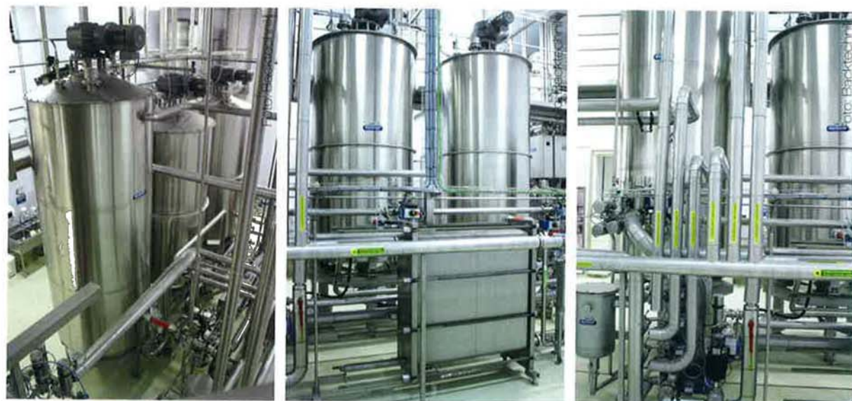
Left photo: The starter dough gets the time to develop in two maturity containers. The big cooled storage tank is on the left. Middle photo: Before the starter dough flows into the storage tank, it is cooled down to 5°C in a plate heat exchanger. Right photo: An extensive cooling system ensures that the individual ingredients are at the desired temperatures.
