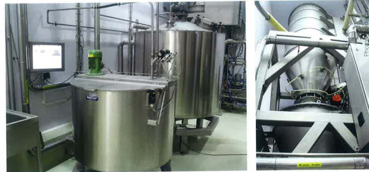
Left photo: At first, the yeast is dissolved and after that, it is pumped to the storage tank next to it. Right photo: While the flour is continuously filled to be mixed in the lower scale, the next batch can be weighed in the upper scale.
