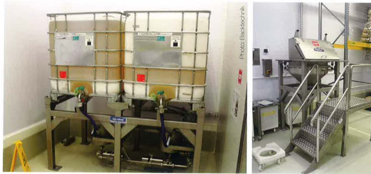
Left photo: Two tanks provide for the sufficient oil quantity that is transported via a pump to the dough preparation unit and the kneader. Right photo: The small-quantity ingredients as well as flour and sugar must be sieved prior to processing to exclude pollution.
