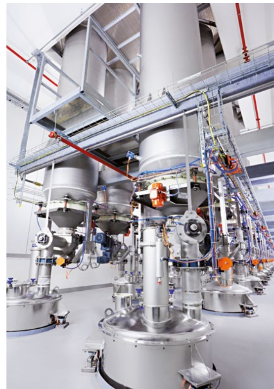
Daily silos with vibro-bin-discharger, weighing bin 500l, Hygienic Design, electropolished for high weighing accuracy
