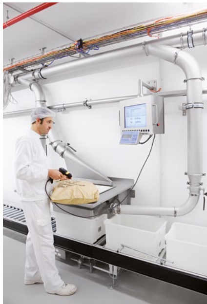
Bag dumping into PU-troughs, storage in automatic storage and retrieval system for small and micro components
