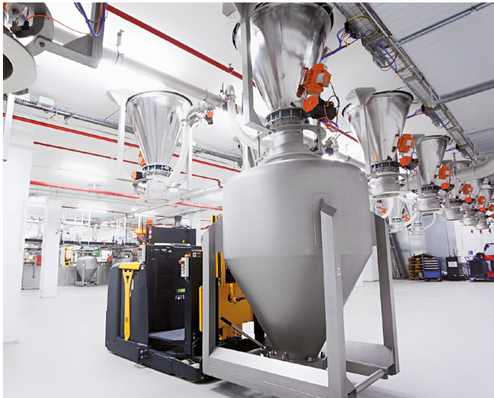
Automatic Guided Vehicle (laser-guided) with Daxner Container Hygienic Design DCHD
