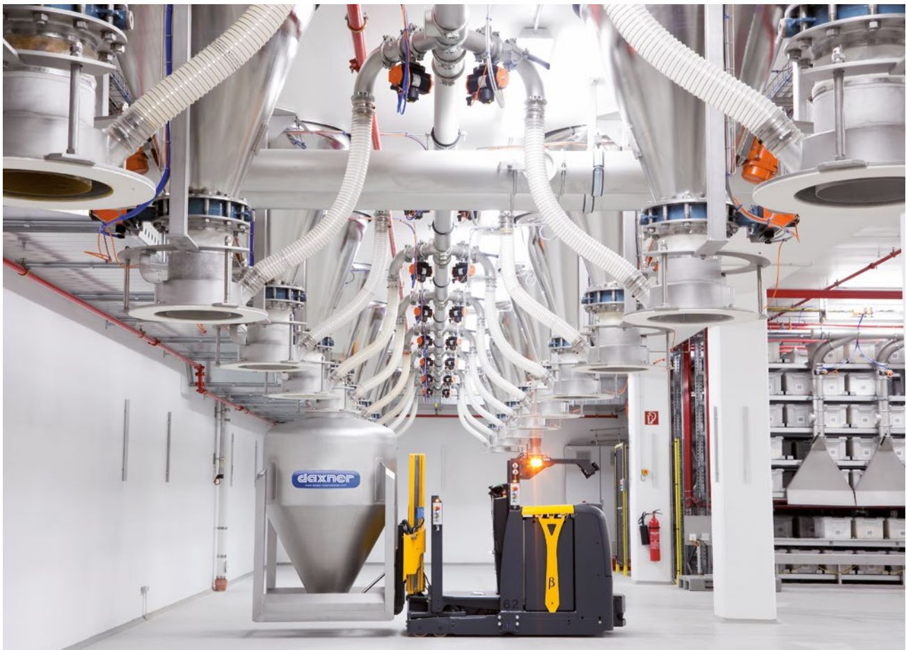
Fully automated collection system with Daxner Container Systems DCS and AGV (Automatic Guided Vehicle)
