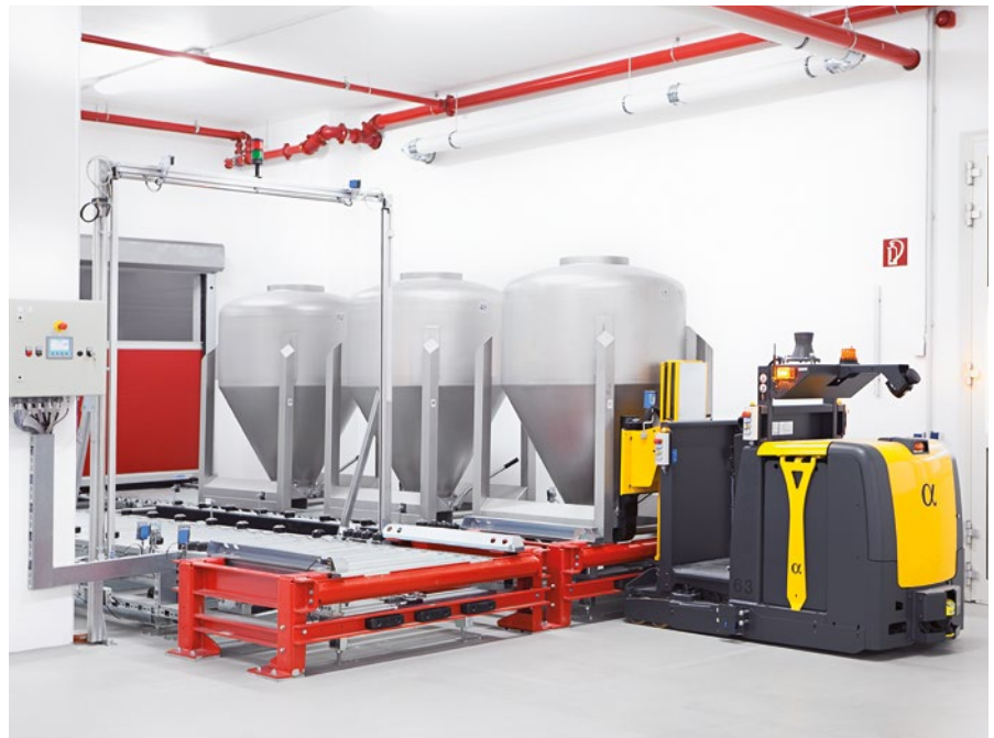
IBC transport system on roller tracks and with lifting device
