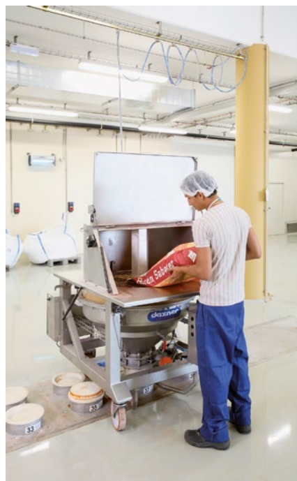
Intake of raw materials with the mobile bag dump station VIB & PRESS with stirring paddles and control screen
