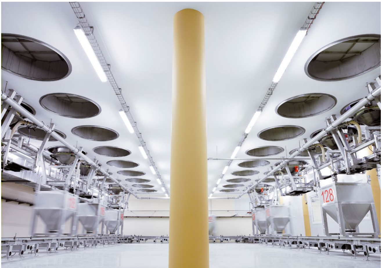
An IBC handling system with cover-manipulator collects the dosed and weighed components
