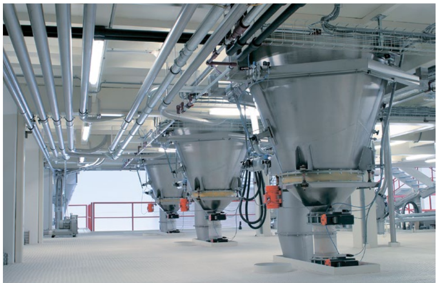
Weighing bins with vibro bin dischargers.
