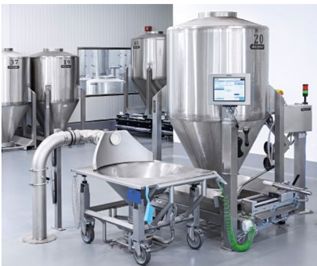
Container discharge with automated flap opener; mobile bag intake station
