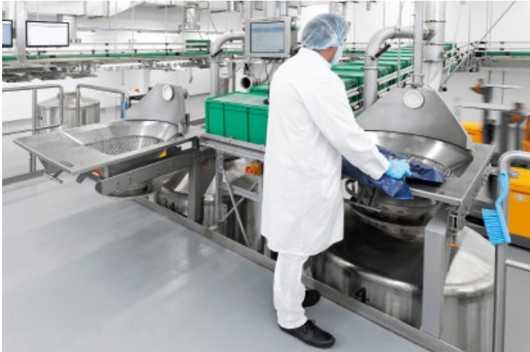
After collecting the automatically dosed components, the container is positioned under the manual loading station. This is where all small components get loaded in complete bags and/or as a subset from the automated storage and retrieval system.
