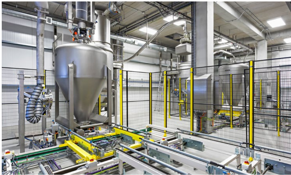
IBC transport and discharge system above mixing level
