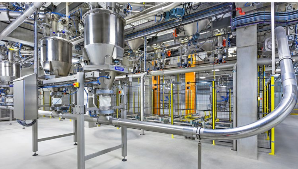
High accuracy dosing and weighing of bakery ingredients including vacuum transfer system
