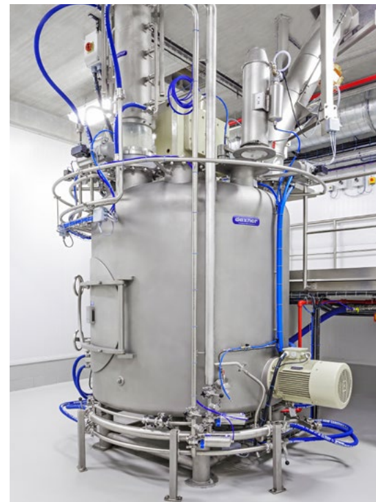
The CIP-able blender ensures highest mixing accuracy (1:100.000) for powder mixes inclusive the addition of block fat resp. liquid fat.
