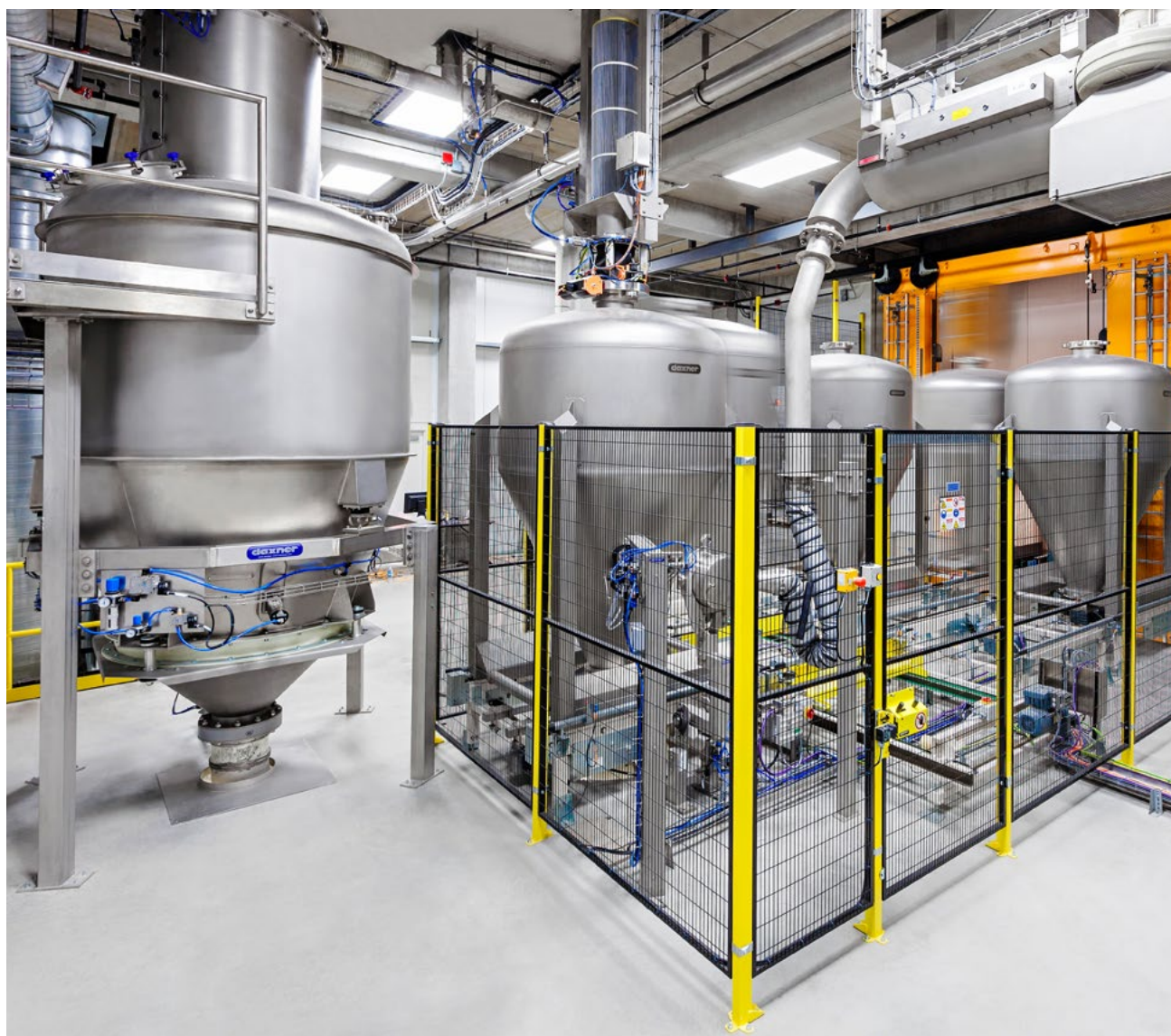
Fully automated mixer feeding through receiver bins (outdoor silos) and a three-dimensional container transport system
