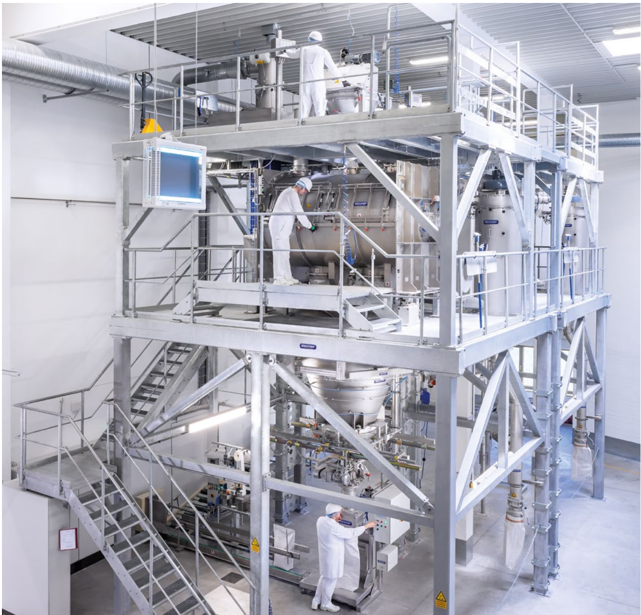
Company Katech assigned Daxner for the planning, delivery and installation of a gravimetric, compact designed mixing plant equipped with two separate mixing lines
