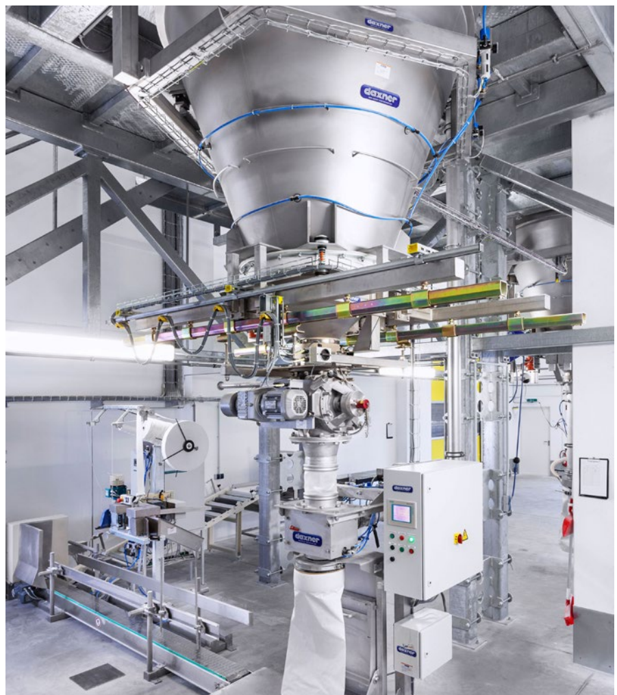
The gravimetric bag filling and weighing system of the series DAX-PVS fills the finished mixes into bags
