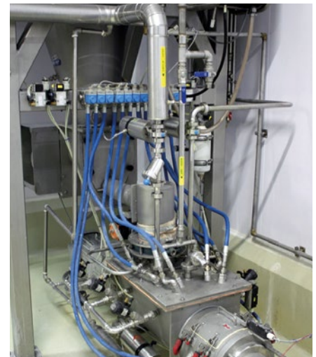
Flour, water, yeast, and oil are mixed in the dough preparation unit and then are pumped into the maturation container.
