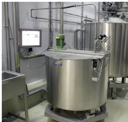
At first, the yeast is dissolved and after that, it is pumped to the storage tank next to it.
