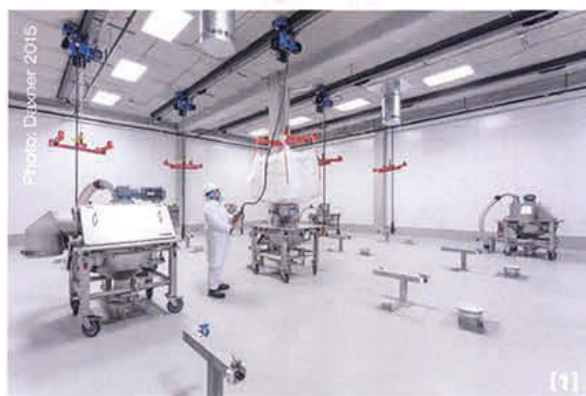
[1] Medium components are stored in day silos and filled by mobile feeding stations with integrated control screening machines. [2] Large components are stored in external silos and pneumatically fed to the mixing lines.
