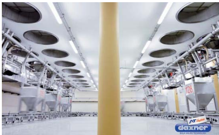
Dosing of raw materials with dosing screw and weighing vessel
