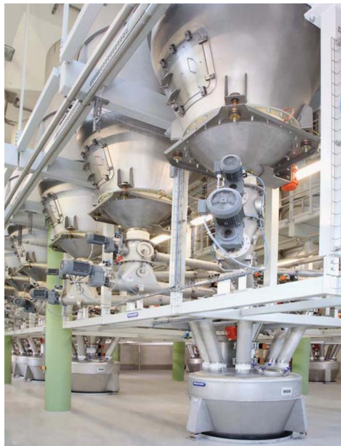
An IBC handling system with cover manipulator collects the dosed and weighed components
