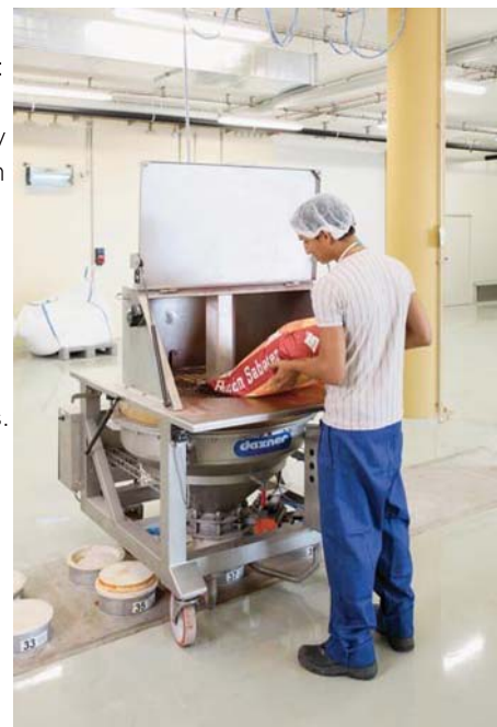
Intake of raw materials with the mobile bag dump station VIB & PRESS with stirring paddles and control screen
