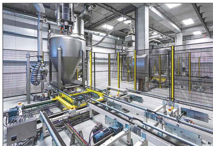
Daxner installed a fully automated mixer loading system through suction vehicles for the external silos and a three-dimensional IBC transport system.
