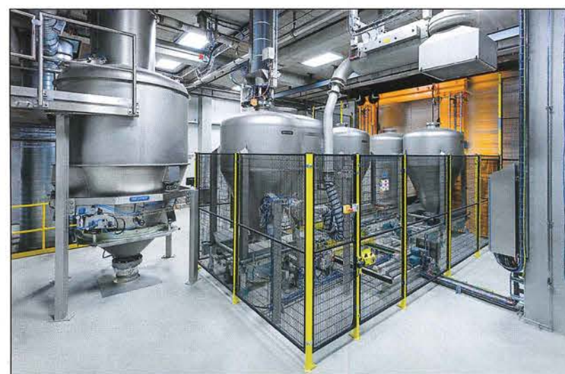
Fully automated mixer feeding through receiver bins (outdoor silos) and a three-dimensional container transport system.
