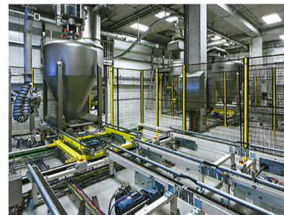
Daxner installed a fully-automated mixer loading through suction vehicles for the external silos and a 3-dimensional container transportation system
