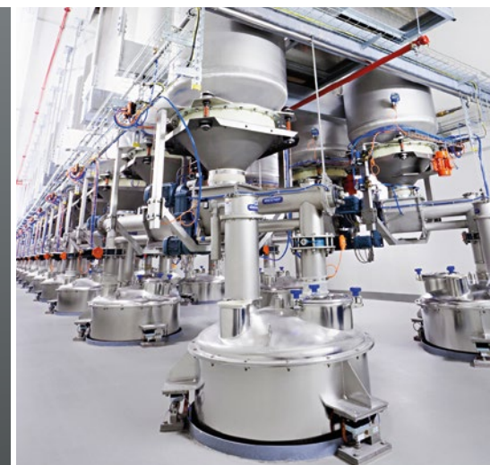
Precision dosing of small and medium components out of daily silos
