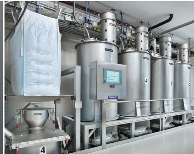
Combined bag intake & bulk bag discharge station together with daily silos for medium components
