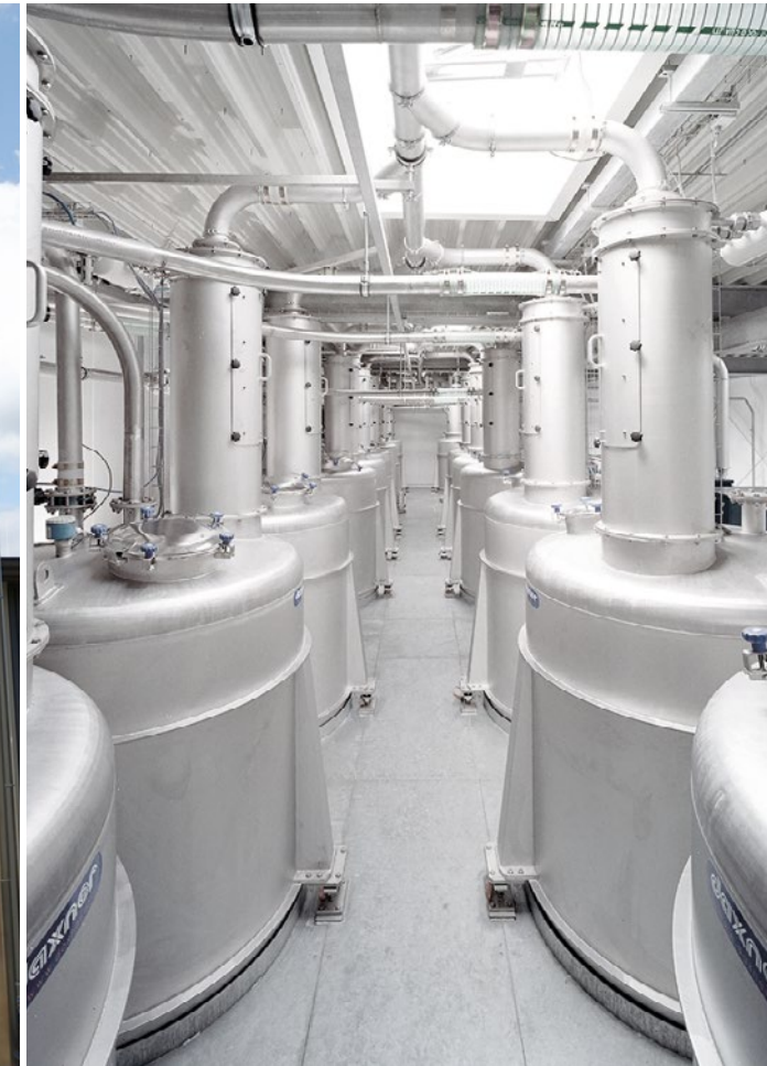
Components such as milk powder, sugar, starch etc. are stored in rounded daily silos
