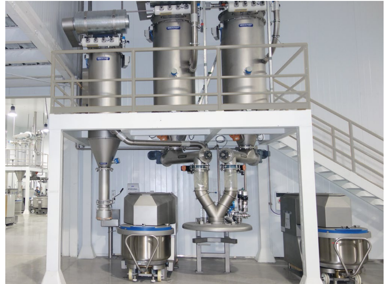
Automated kneader feeding including a loss-in weight dosing system
