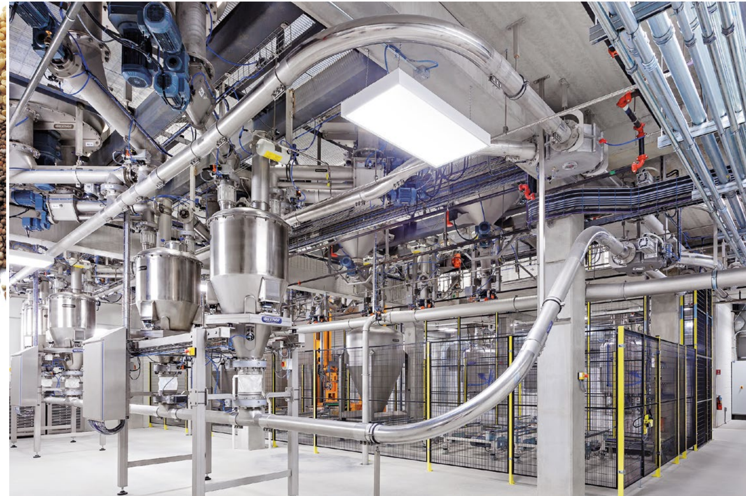
Pneumatic vacuum conveying system in combination with DCS Daxner Container Systems
