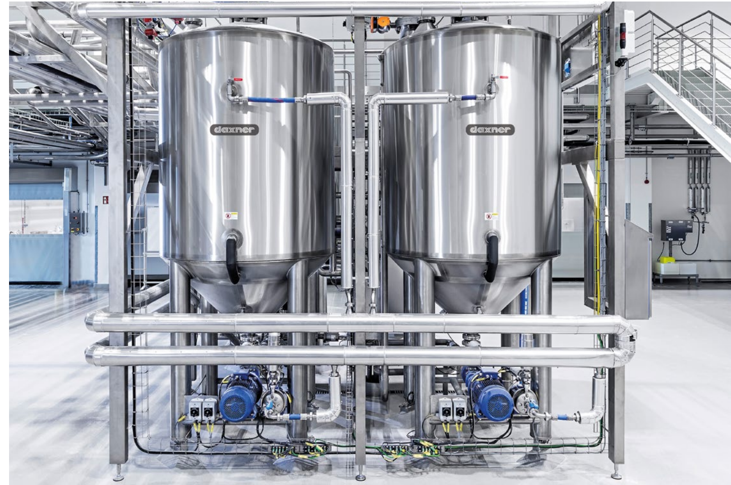
Fermenter for all sour and pre-doughs - Design with pig cleaning system for both product discharge and a clean separation of consecutive batches
