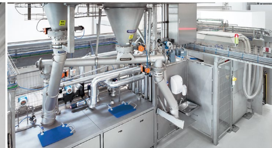
Fully automated kneader feeding with powders and liquid ingredients
