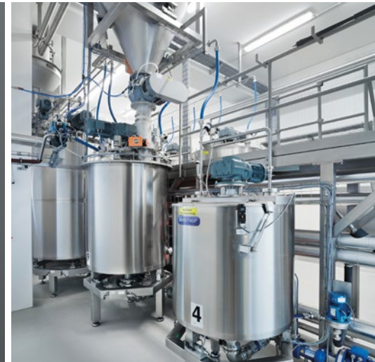
Sourdough starter and fermentation tank for wheat sour dough
