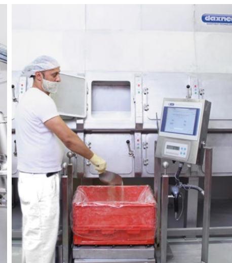
Operator guided manual dosing system for small and micro ingredients
