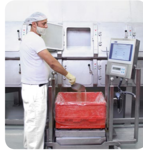
Manual dosing station
