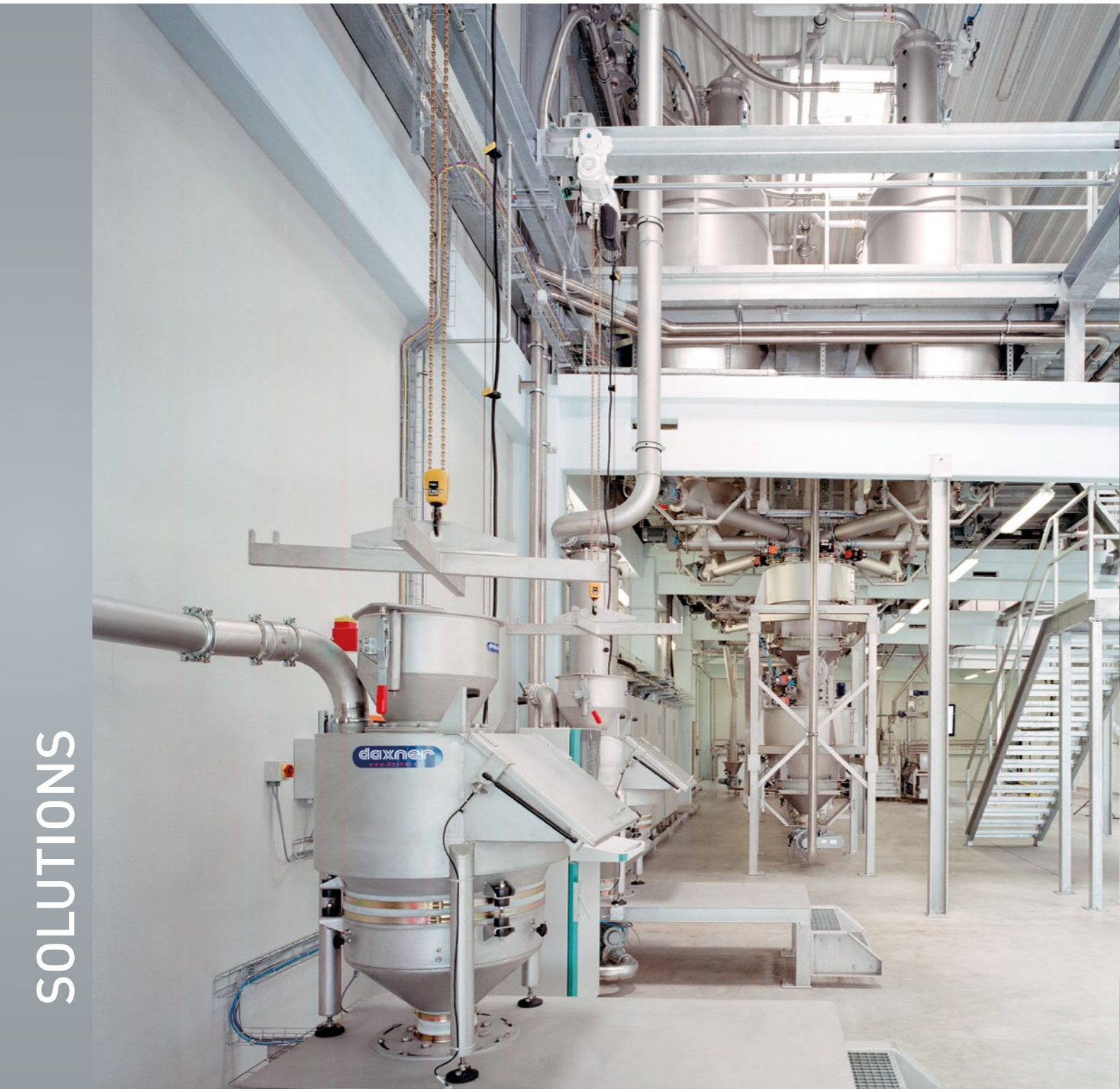
Processing facility for the production of masses for the cookie and waffle manufacture. Hygienic handling of high-quality raw materials fed out of bags or Big Bags. Liquid ingredients are dosed by dosing pumps through heatable pipes. The plant and dosing controls system ensures a seamless traceability of all components and batches.
