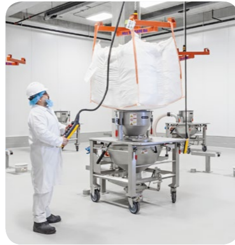
Big Bag discharge station
