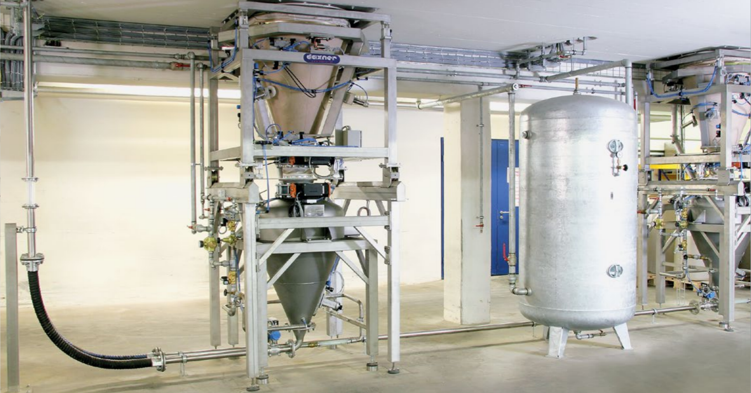
Automatic batch component dosing facility for mineral additives. The handling of ingredients with poor flow characteristics imposes highest requirements on the IBC System. A flexi-scale and a pneumatic dense phase conveyor are essential key components for this sophisticated system.
