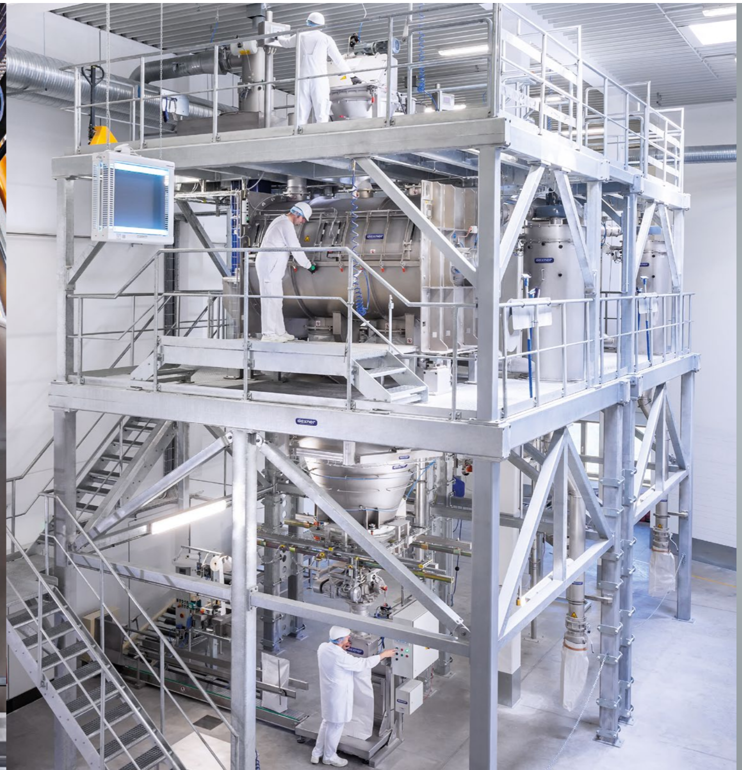
Compact designed mixing plant for the production of complex bakery ingredients. An efficient plant design ensures flexibility for product changeovers with utmost mixing accuracy. High-end product quality can be achieved due to the prevention of cross contaminations by featuring hygienic design and easy cleaning.
