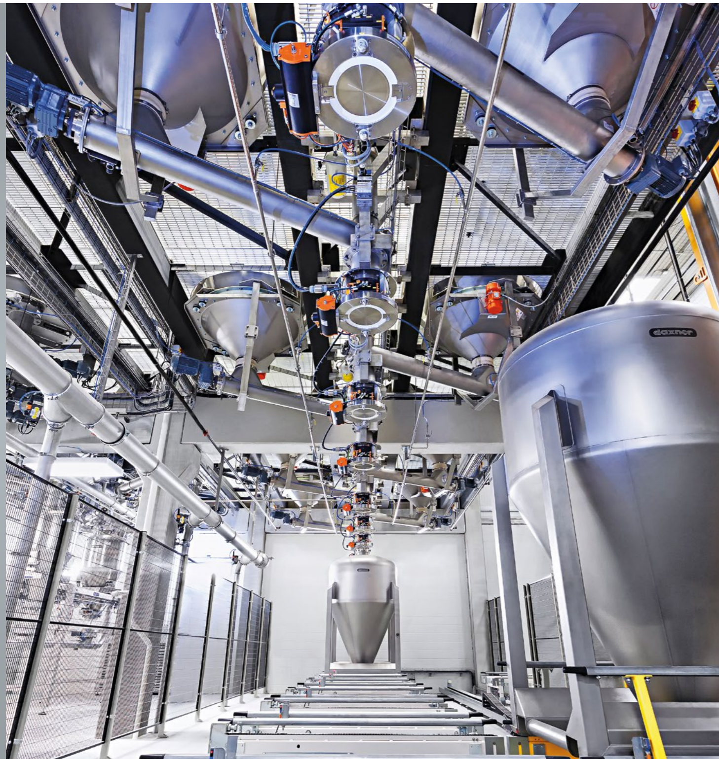
Uncomprising hygienic design in a bakery ingredient mixing system. A fully automated three dimensional container transport system provides for high throughput, dosing accuracy and allergen-free ingredient handling. A full CIP-able mixing tower minimizes cleaning downtime and maximizes operational efficiency.
