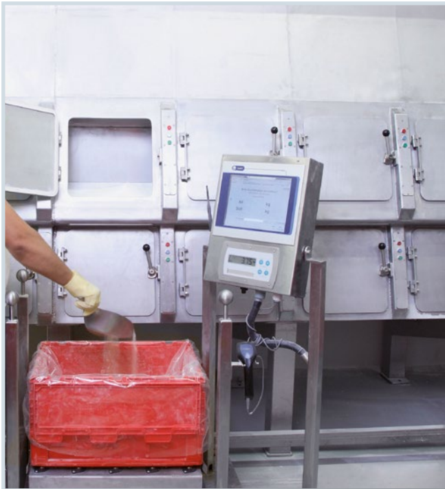
Picture: Small Component Bins with hinged withdrawal opening and call light (pick-to-light-system); Mobile weighing and dosing station with control station 15", incl. plateau scale; Data transfer with WLAN
