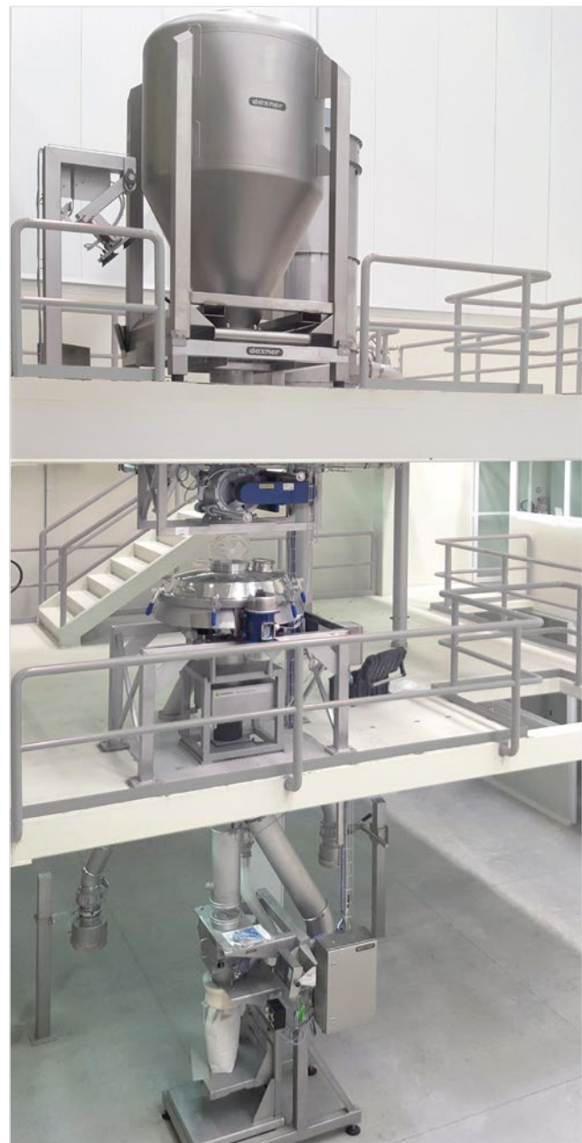
Complete view of the mixing line: controll screening machine, VIB&PRESS, big bag product intake station, mixer, IBC docking station sowie IBC container
