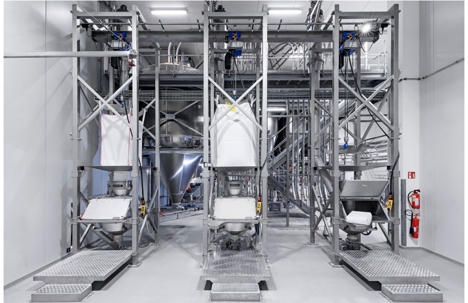
Big bag station with integrated bag intake including sieving and metal check for filling day silos.
