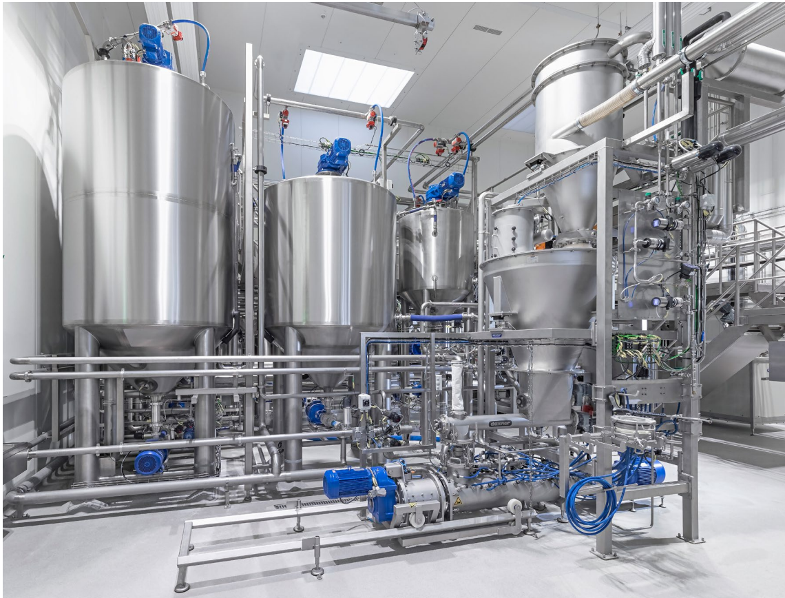
Sourdough system with continuous mixer for homogenous blending of flour and water
