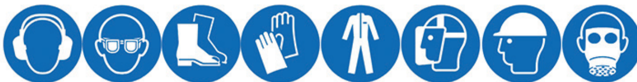
hearing protection eye protection foot protection hand protection protective clothing face protection safety helmet respiratory protection
