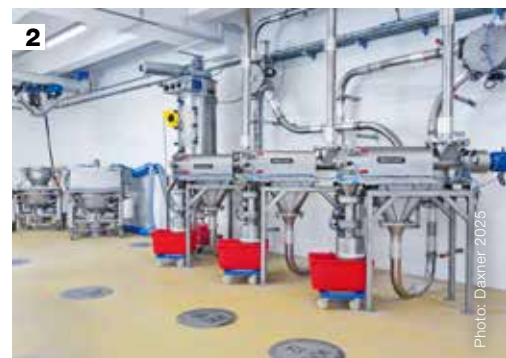
1 The automatic medium component system is equipped with a weighing and conveying system. 2 Inline sieving machines with bag chutes and big bag emptying station are available for the efficient filling of the ingredient silos.
